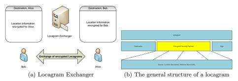
Fig. 1. Communication is done using a common known locagram exchanger
