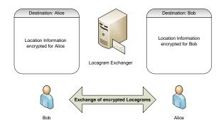
Figure 1. Communication is done using a common known locagram exchanger
