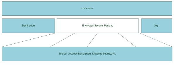
Figure 2. The general structure of a locagram
