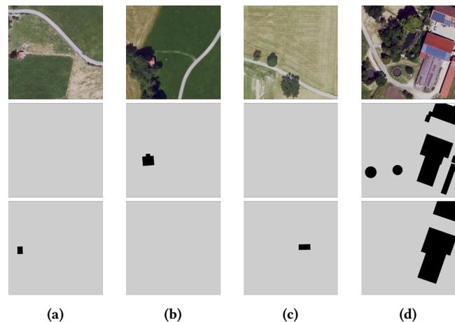
Figure 3: Examples: (a) Missing in Official, (b) Missing in OSM, (c) Missing in Orthophoto, (d) Semantic Difference (Top: Orthophoto, Middle: Official building footprints, Bottom: OSM)
