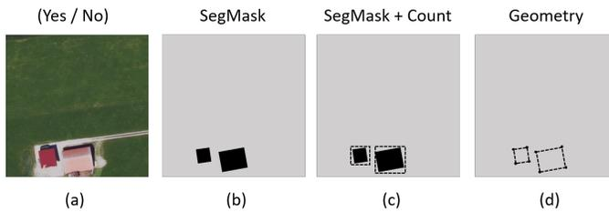
**Figure 4: Exemplary analysis tasks with the BBD dataset: (a) Detection, (b) Segmentation, (c) Instance Extraction, (d) Footprint Geometry Extraction.**
